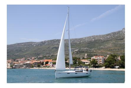
**Destination:** Croatia Base: Split Length overall: 13.85 m Beam: 4.49 m **Draft:** 2.15 m **Guest Cabins:** Guests number: 10 Berths: 8+2 Showers/toilets: 2 Engine: 54HP Fuel tank: 200 L Water tank: 570 l Year built: 2012 Manufacturer: Beneteau
